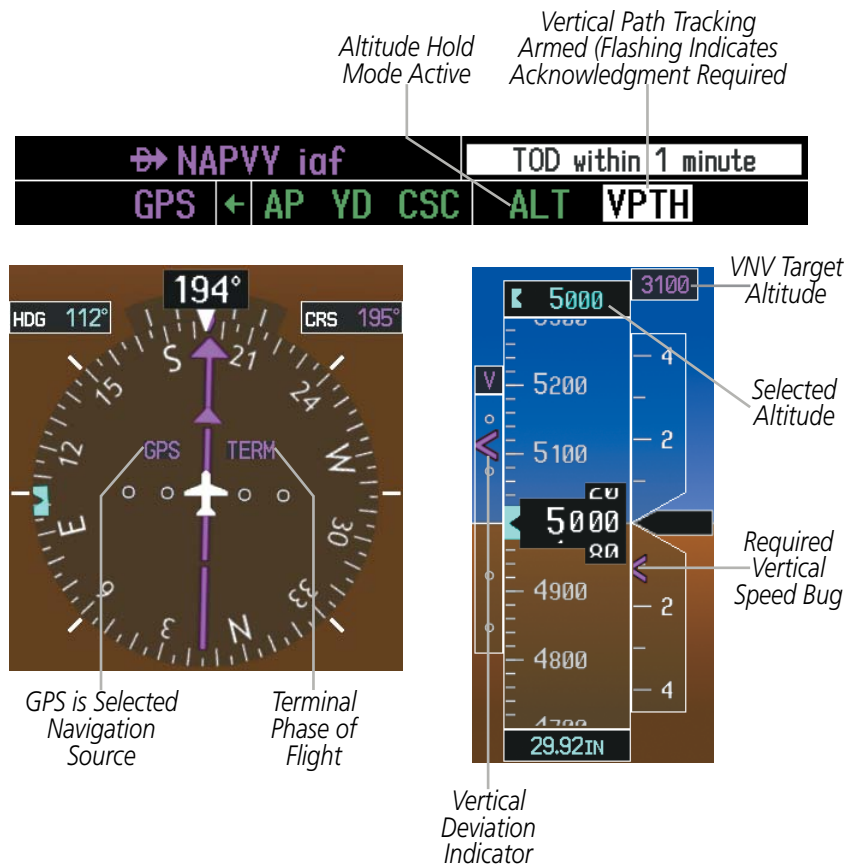
Figure 7-14 Vertical Path Capture
